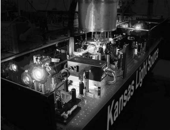
Figure 1.2 A femtosecond high-power laser system. The whole laser fits on one 8' \times 12' optical table. The cylindrical container above the laser beam is for cooling the laser gain medium with liquid nitrogen.
